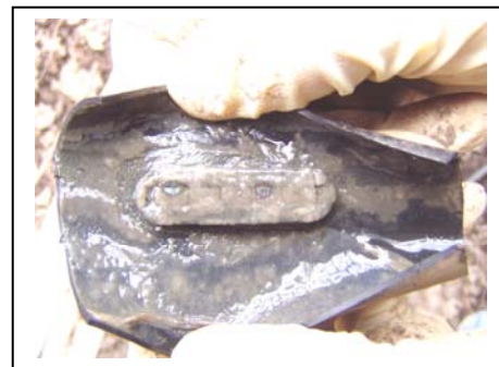
Figure 3 – Drip irrigation emitter with extensive bacterial growth, plugging the emitter.
